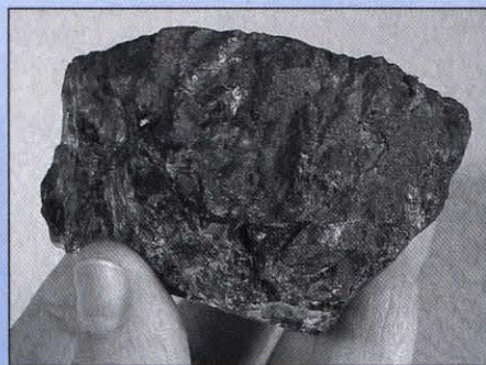
Figure 12 Stinkspat specimen from Wölsendorf, Germany. When ground in the presence of starch/KI paper, a blue color develops, showing the presence of a strong oxidizer (F 2 inclusions).
